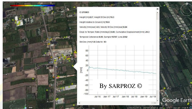
Figure 27 The result of PSI215903 by SARPROZ software on the Google Earth background.
