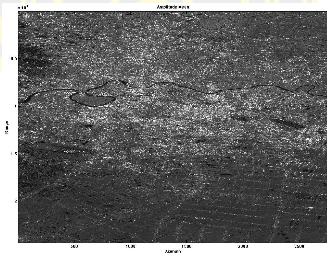
Figure 8 The mean of the amplitude map in ascending orbit using PS-InSAR techniques by SARPROZ software. (The grey colours range represents a backscattering strength.)
