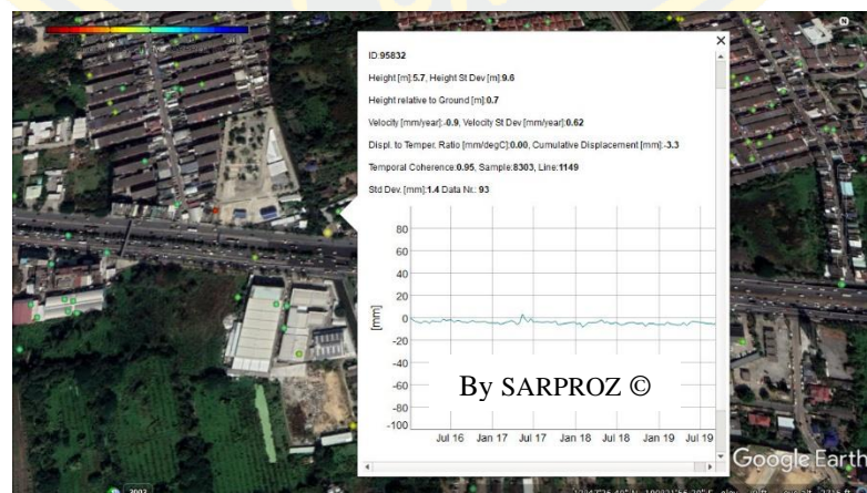
Figure 29 The result of PSI95832 by SARPROZ software on the Google Earth background.
