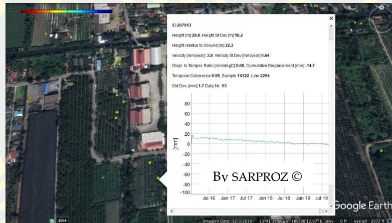
Figure 28 The result of PSI207913 by SARPROZ software on the Google Earth background.
